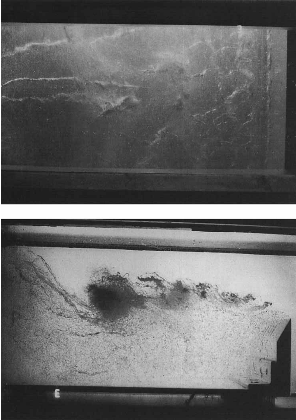
FIGURE 7. Simultaneous top and side photographs of well-developed cavitation in the shear layer. U_L = 10.14 m/s, \sigma_L = 0.39 , Re_L = 1.84 \times 10^6 .
